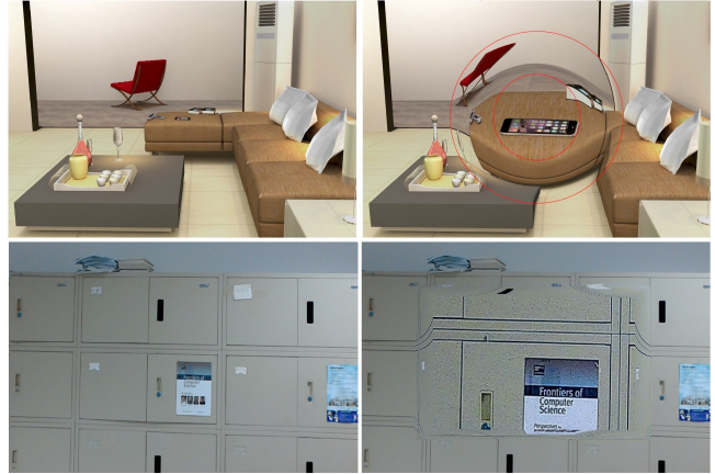
Figure 1. Top: conventional (left) and our focus+context (right) visualization in VR. The focus region (inner circle) has a distortion-free 5x magnification factor, and it is connected with C^1 continuity to the surrounding context. Bottom: conventional user view (left) and our AR focus+context visualization (right). The AR HMD is enhanced with a high resolution camera that provides the magnified view of the real world, which is integrated continuously into the user's view.
