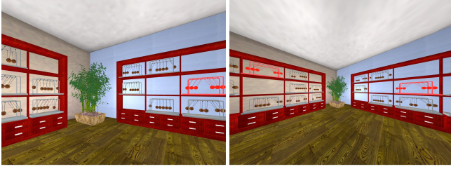
Figure 2. A conventional VR visualization that uses the HMD's natural field of view cannot show both shelves at the same time (left). Both shelves are visible when the user zooms out, and the red-highlighted cradles with identical motion pattern can be matched (right).
